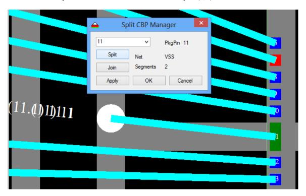
After fanout has been executed again you will see that the 2 segments have been fanned out based on the DRC rules set in the Tiers Properties dialog box. Now the 2 CBP attach points have to be separated.
