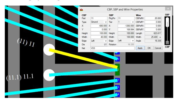
Next select the second segment and set the CBPoffX to -20 and click the Apply button and the CBP wire attach point is moved 20 microns to the left (down in this case).
