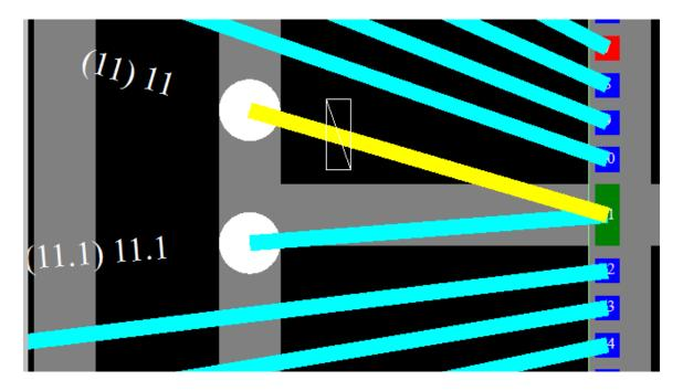
Open the Pad Properties dialog box and the selected wire information will be displayed. In this case I entered 20 into the CBPoffX box and pressed enter to accept the value. Then clicked on the Apply button. As you can see the CBP wire attach point has moved 20 microns to the right. (upward in this case). Remember the offsets are based on the view at the right of the dialog box.
