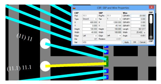
The result of this is pad 11 now has two wires attached to it. (11) 11 and (11.1) 11.1. Since this is in a pad ring you might reduce the Pad to Pad DRC rule for that tier for a tighter design. This depends on the bonding house and what their wire to wire rules are.
